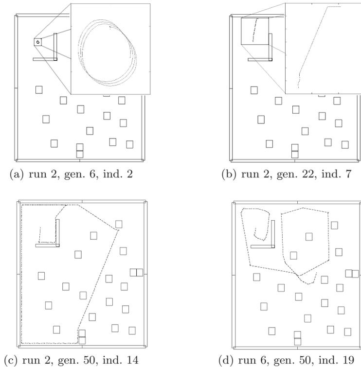
**Fig. 4.** Trajectories of the robot of run 2 (a, b and c) and 6 (d); gen.: generation number, ind.: number of the individual in the population.
