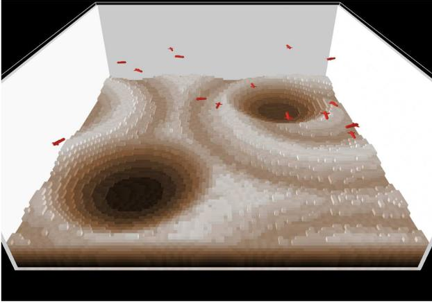
Fig. 2. Screenshot of the experimental arena and its starting conditions. The red objects are AUVs. The two depressions in the ground represent the aggregation spots whereby the left depression can be considered to be the optimal spot for aggregation. At the beginning of each experimental run the AUVs were spawned at random positions.
