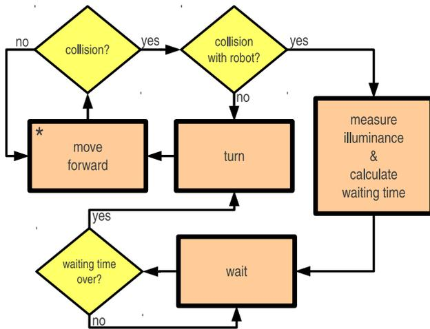
Fig. 1. Finite state machine of the BEECLUST controller. The asterisk indicates the starting state of the algorithm. Please note that the experiments in this work were performed with a depth sensor and therefore we measured the depth instead of the illuminance.
