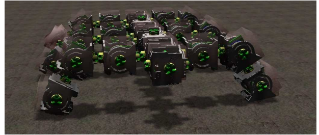
Fig. 1. A possible configuration of robot modules as envisioned in the projects Symbion [3] and Replicator [4] using the Symbicator3D simulation [5], [6].
