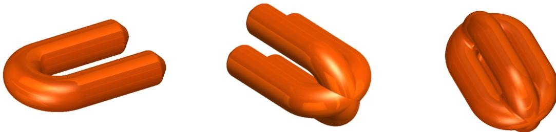
Figure 1: Concepts of CoCoRo AUV shapes with different abilities for the resulting AUV swarm. Each of these small AUVs will be equipped with multiple sensors to allow them to be aware of their environment and their swarm members. Images
