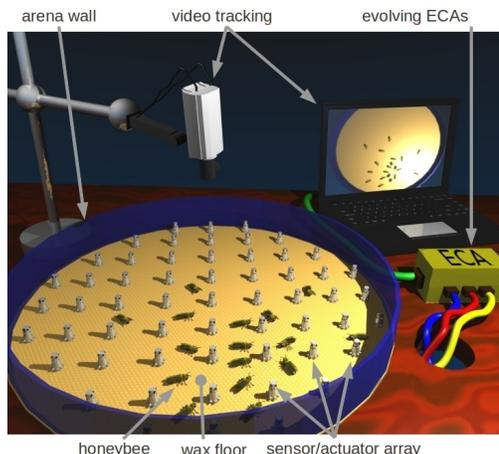
Fig. 1. Computer artwork demonstrating the planned experimental setup with honeybees and autonomous devices (CASUs) in ASSISI<sub>bf</sub>.
